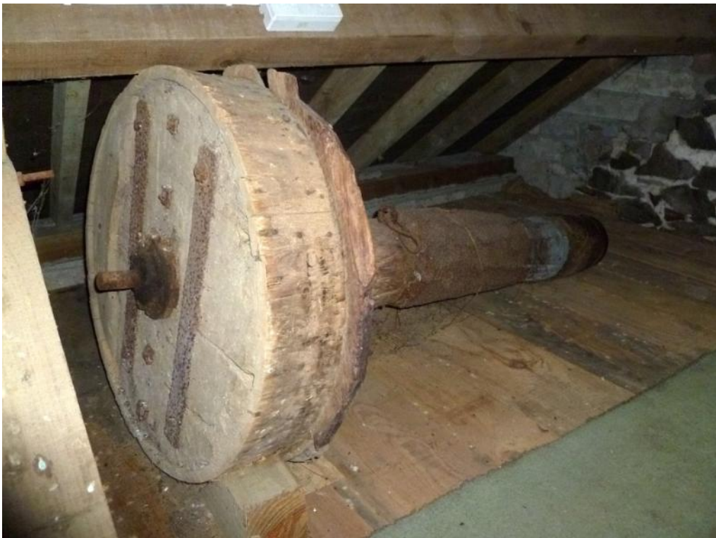
Sack hoist chain bollard drive pulley
