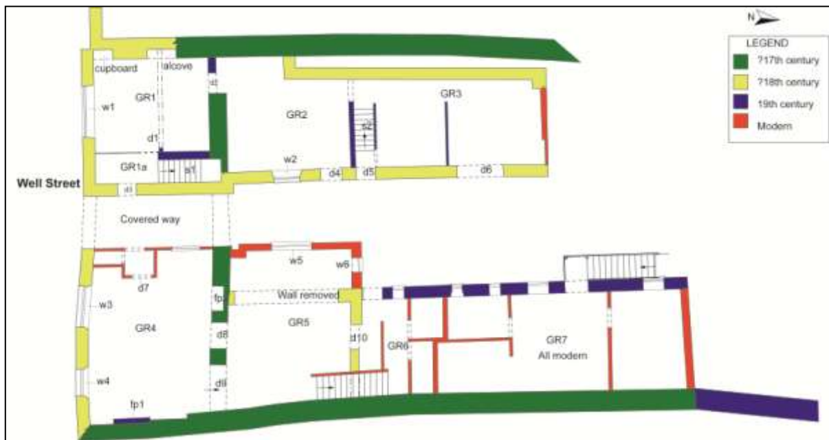
FIGURE 9: PLAN OF ADMIRAL VERNON/NEW INN SHOWING ROOM LOCATIONS AND FEATURES DESCRIBED IN THE TEXT.
