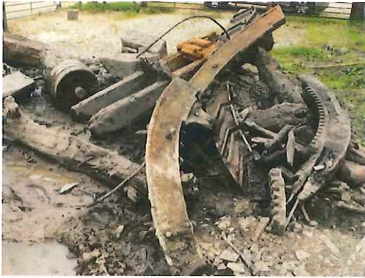
Remains of waterwheel and gear ring
