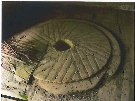
Conglomerate millstone, 1st floor
