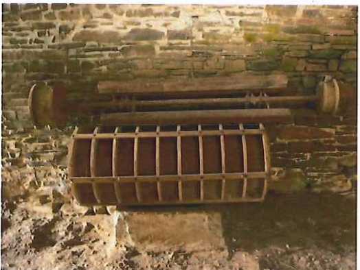
Cylinder and shaft of corn cleaner
